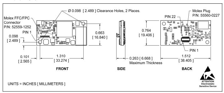
Figure 11. TTL Level RS232 Decode Board
